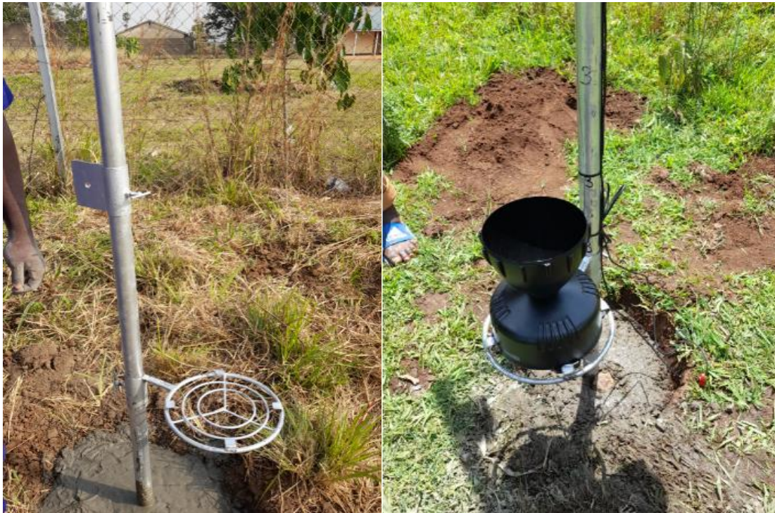
Figure 4.4: Fixing the rain gauge base on the stand close to the ground
