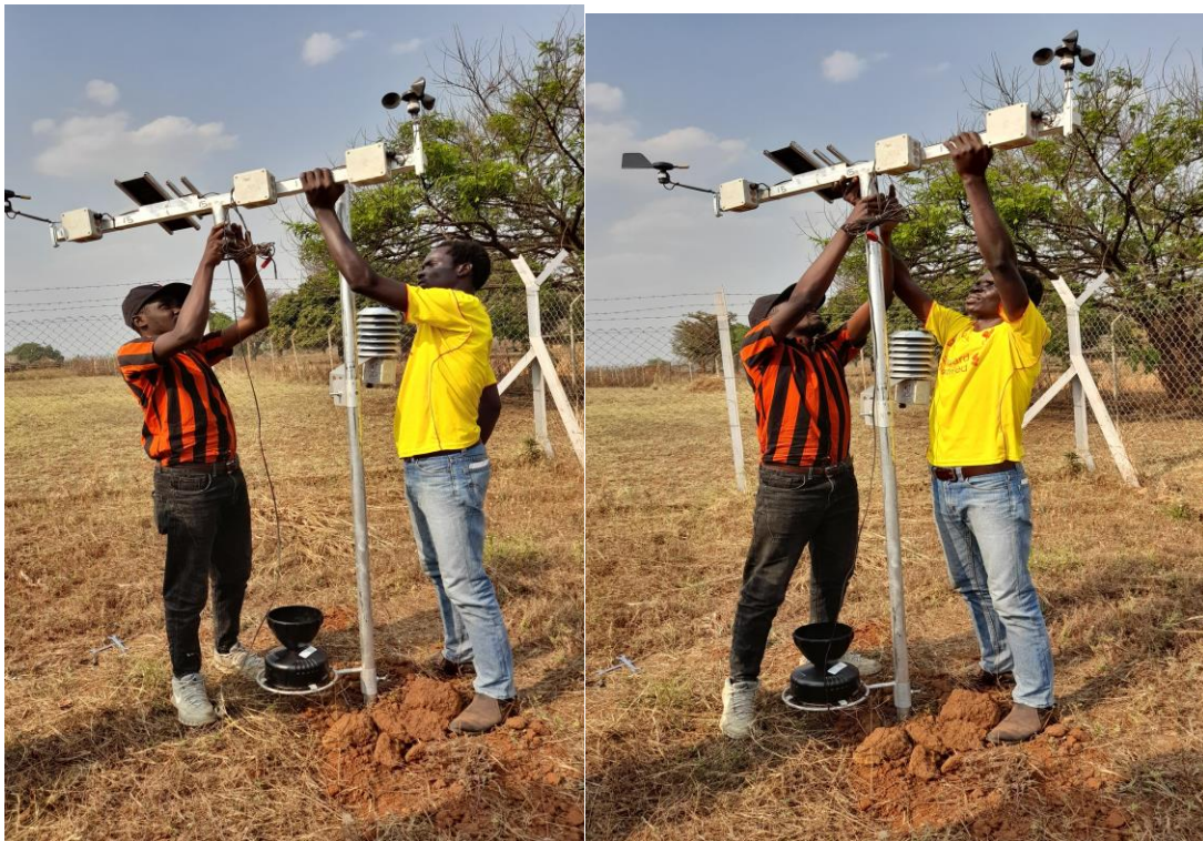
Figure 4.6: Attaching the top part of the stand
