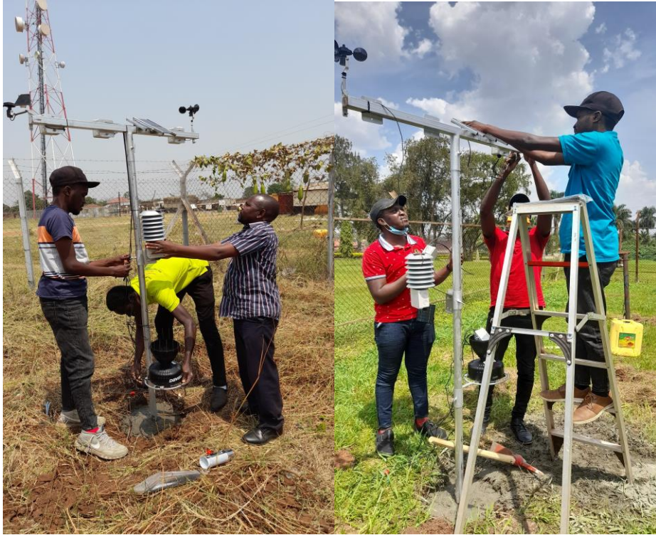
Figure 4.7: Adjusting and fixing the soil and wind sensors and rain gauge
