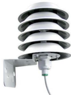
Figure 2.7: The 2m node's Radiation Shield
