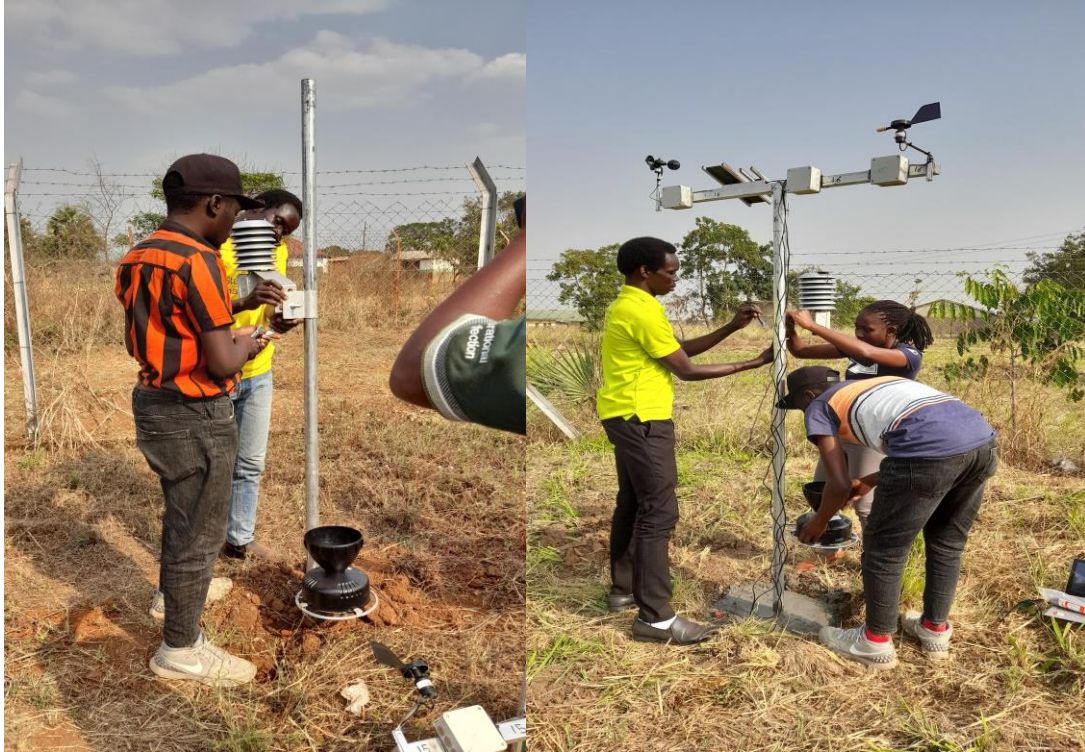
Figure 4.5: Attaching the 2m node on the stand and adjusting to the right position
