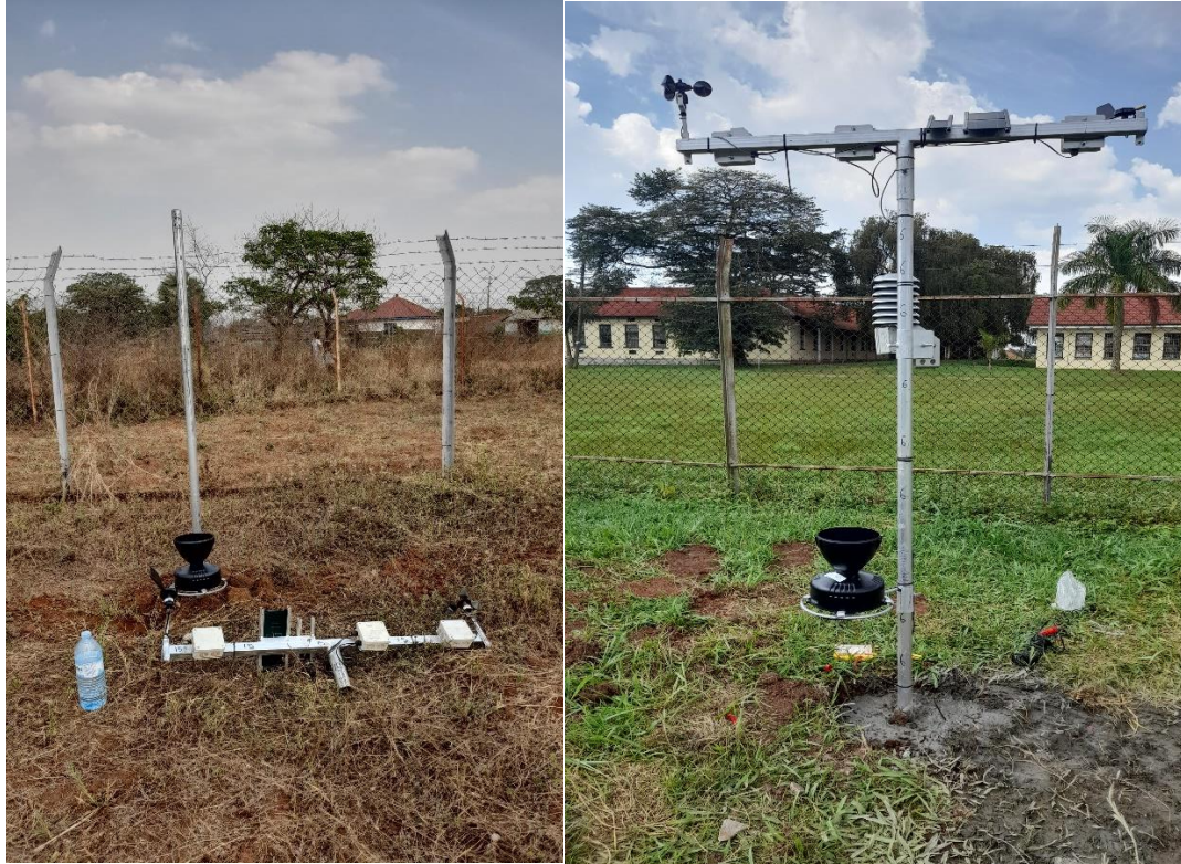
Figure 2.6: The New design of the AWS Stand
